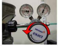
5- Shut the compressed air bottle (silver pressure regulator) and the CO2 (golden pressure regulator) by turning them in clockwise direction.
